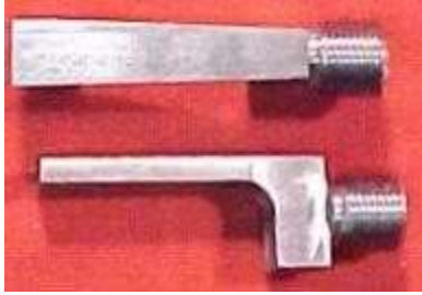
Figure 4a: Breech plug and Tang both require a gunsmith to be removed from the barrel of the pistol shown above.
